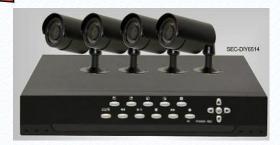
DVR: H.264, 4CH/120fps, VGA & BNC output, USB2.0 Backup, Remote controller, Mouse, Network (DHCP, DDNS), Mobile Surveillance
